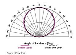
At first, it would seem logical to plot a cosine response on a polar plot (Figure 1). However, the polar plot only shows the general shape of the response which is good for a quick visualization. It does not show details of the error to a perfect cosine response. Errors of a few percent are nearly impossible to see on a polar plot. Therefore a Cartesian system with the error curve shown is a better choice (Figure 2).
