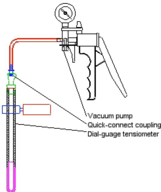
into the tensiometer tube through the porous cup, filling the pores and replacing the air in the cup with water. When the reservoir tube is completely filled with water, the vacuum pump is removed, and the tensiometer is removed from the container of water.
