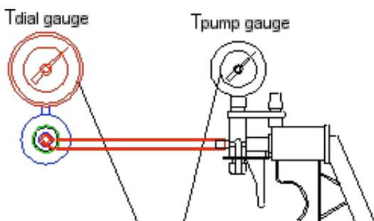
offset =  $T_{\text{pump gauge}} - T_{\text{dial gauge}}$
