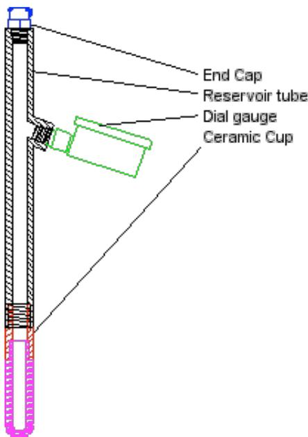
The tensiometer consists of several main components: a porous ceramic cup, a water reservoir tube, a dial gauge, and an
