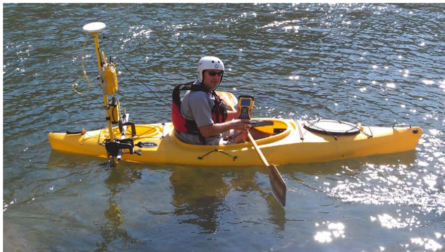
Figure 7. Photograph of kayak based bathymetric survey setup.
