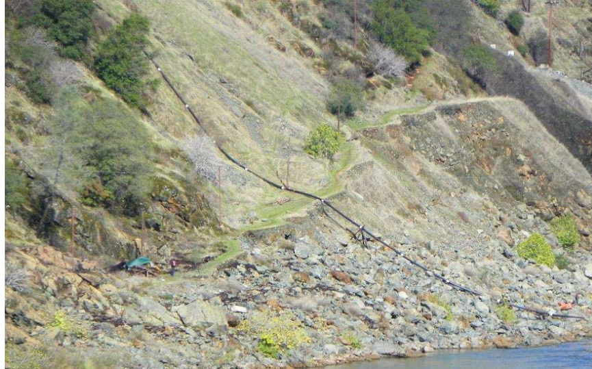
Figure 1. Gravel/cobble sluice pipe and temporary lean-to. Photo courtesy Ralph Mullican.
