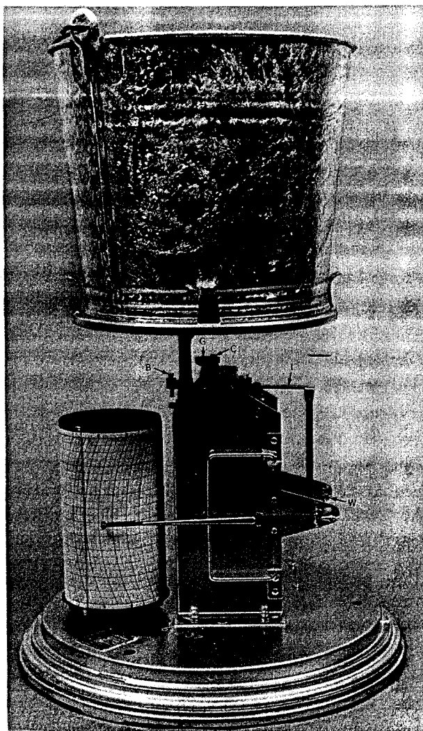
FIGURE 1.13.—Single-traverse rain gage showing the location of some stops and linkages.
