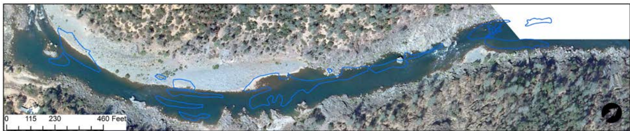
Figure 3. Polygons outline areas of gravel deposition that were discernible using the Google Earth imagery taken in May of 2013 and RTK data collected during the summer of 2013.
