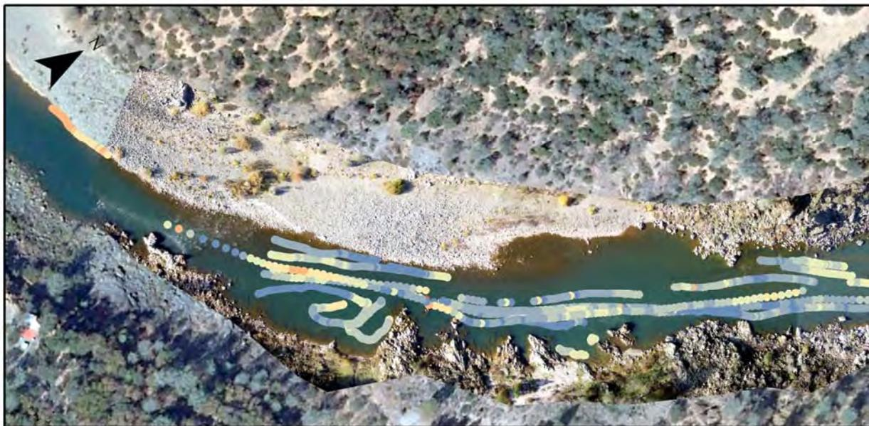
**Figure 18. Spatial plot of observed (with DAVC adjustment) minus modeled velocity deviations. Darker red values are where the model under predicted velocity and darker blue is where it has over predicted. Note that legend is not equally centered.**
