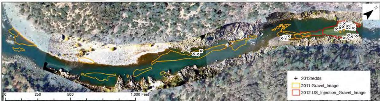
**Figure 47. Observed redds and boundaries for upstream and downstream TCD analysis. Note that the upper cluster is located in the constructed riffle and the middle cluster was outside of the TCD boundary.**
