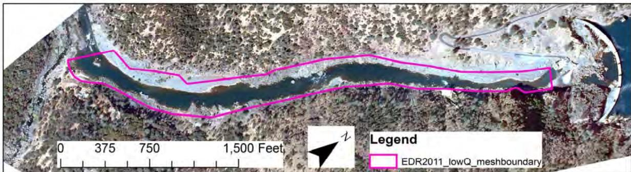
**Figure 9. Extent of EDR 2D model computational mesh for in-channel low flows.**
