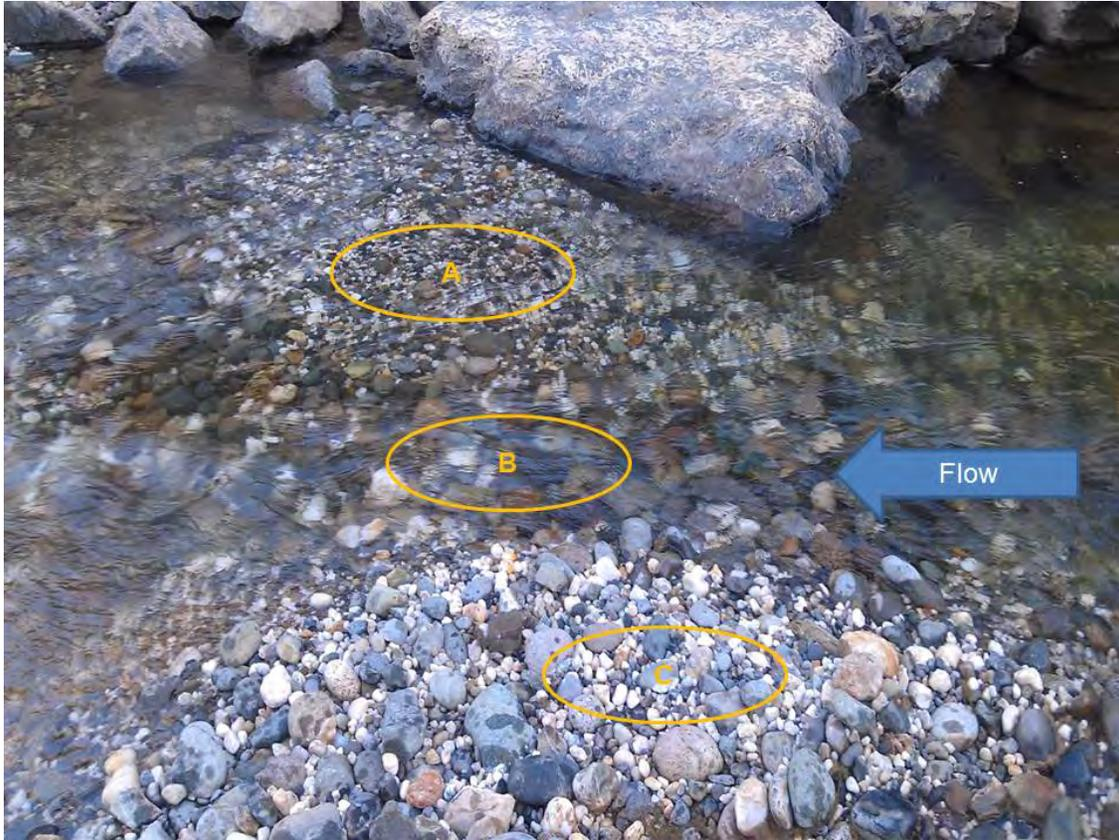
**Figure 12. Photograph illustrating the effect of armoring on injected gravel deposits. When this area was first filled with gravel all areas had very similar grain size distributions but as flow poured through area B this zone coarsened relative to the other areas limiting any further incision.**
